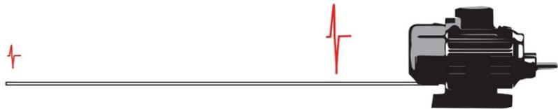
Transient voltages can cause computer equipment to lockup and data to get garbled, or even damage computer equipment. When a transient strikes your computer, it can cause internal noise spikes that may disrupt data. If the transient has sufficient energy, it can cause an arc within the internal components of the computer.
