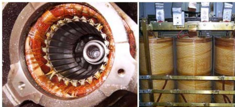
When a transient reaches the coil of a motor or a transformer it will dissipate the majority of its energy in the first few coils. Each successive coil presents more resistance and capacitance to the transient. This will reduce its magnitude and increase its period, reducing the energy. Since the majority of the energy is transferred to the first few coils, this is where the damaged insulation will typically appear.
